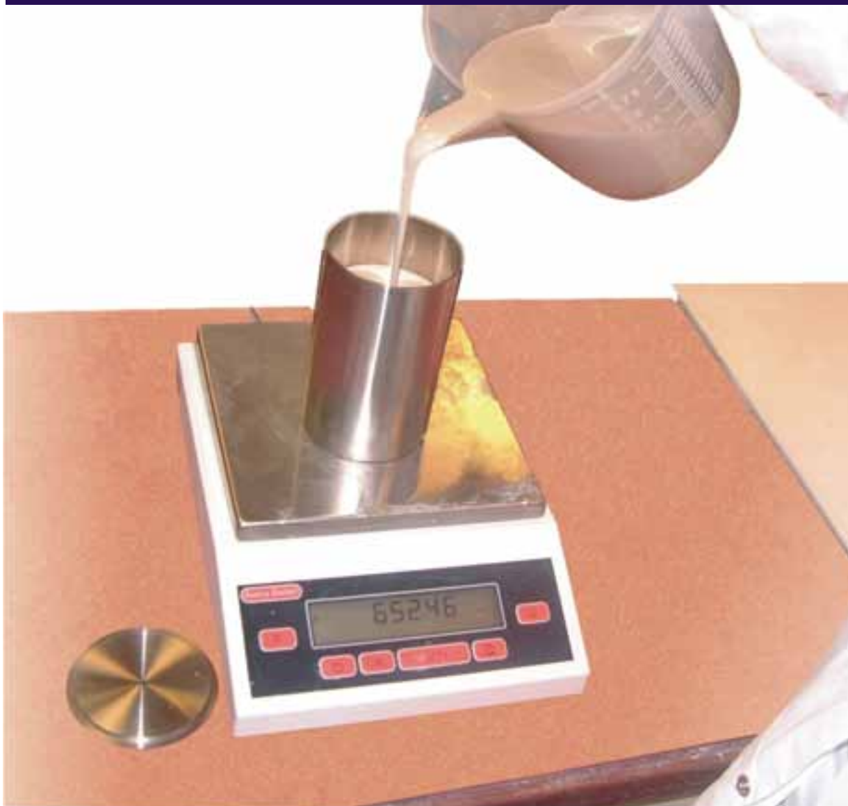
Figure 5: Measurement of Casting Slip Density
