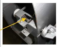
Move the pedal or lever up and down to ensure parts are fully lubricated with the WD-
