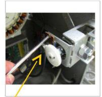
4. When the wheel head stops, slide the potentiometer up against the white gear and tighten the screws down. Then replace the cover 4 feet. Your wheel should now be running from stop to 250 rpm.
