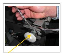
Loosen the first bolt (double nut)
